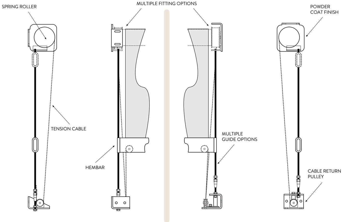
TESS™ systems are built around a unique single barrel tension mechanism. Motor, spring, gearbox and control cable work in harmony to consistently hold fabric flat and intelligently adapt to the surrounding environment, regardless of angle or system direction.
